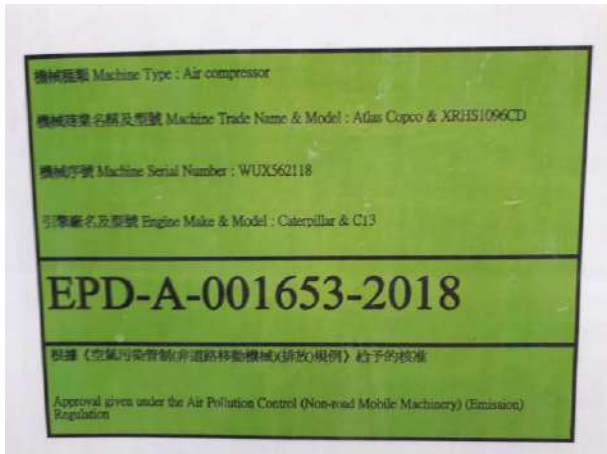
Figure A4 NRMM label on Air Compressor
