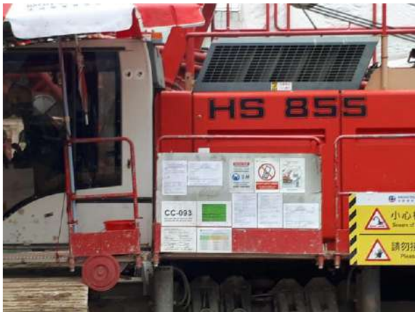
Figure A3 NRMM label on Mobile Crane
