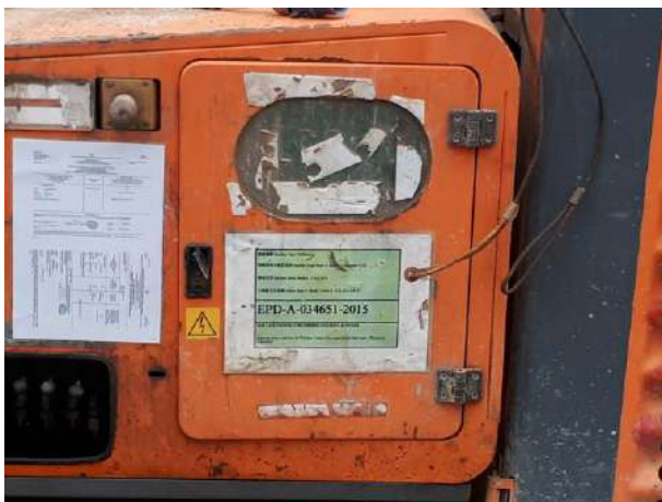
Figure A5 NRMM label on Driller Rig
